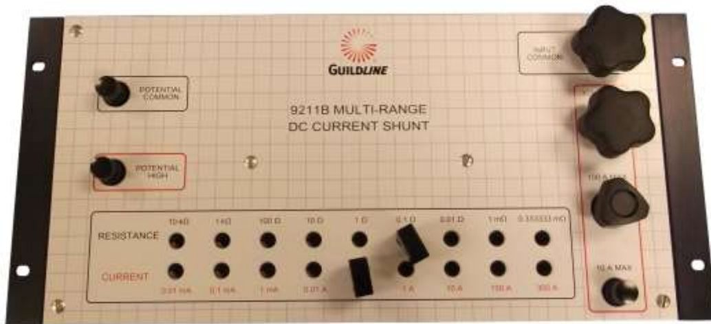
Figure 3-1 : 9211B Current Terminal Connections
