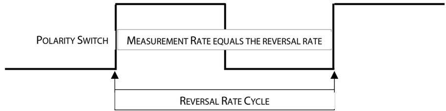
Like all of our new 6640 Series Bridges, Guildline's 6640Q QHR Bridge **decouples the polarity reversal rate** from the measurement rate allowing **measurements to be made much faster** than competitive DCC bridges. As shown in the right figure, you can independently specify a measurement rate and a reversal rate.
